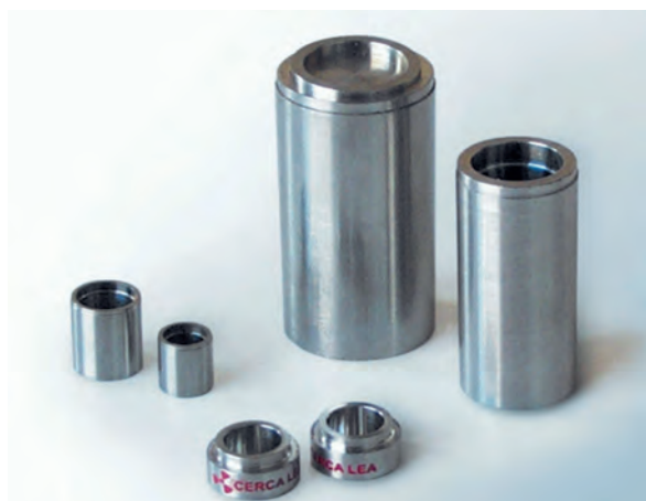
Types de sources scellées gamma
